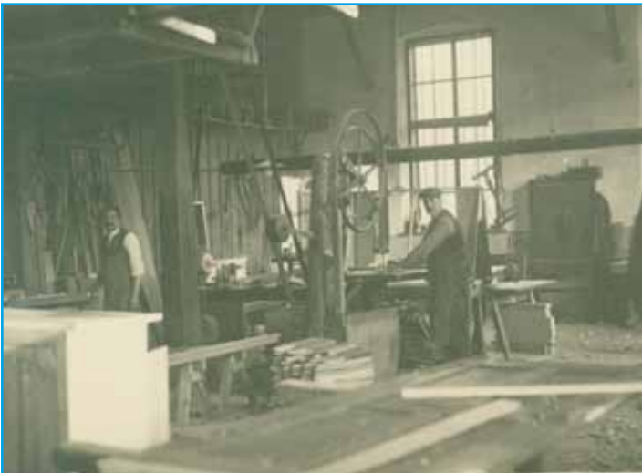
Band-saw in the period of its operation in Francis' shaft.
