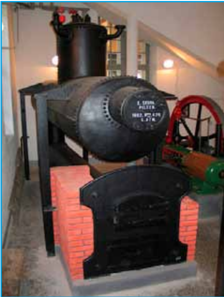
Battery steam boiler as a museum specimen.
